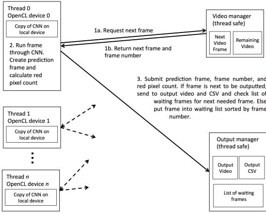
Fig. 4. Overview of the work stealing approach to utilize multiple OpenCL devices to quickly run a trained CNN over a video.
